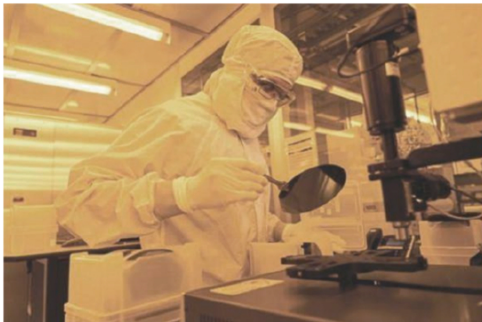
A Rigetti employee inspects a silicon wafer with superconducting quantum integrated circuits that was fabricated at Rigetti's Fab-1 facility.
