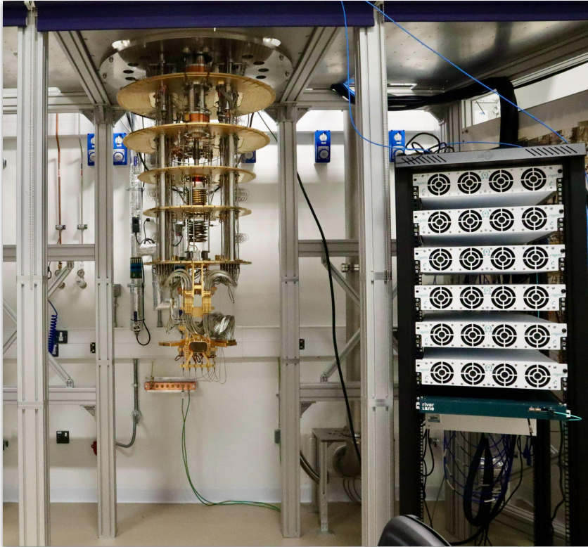
Rigetti's 36-qubit quantum computer hosted at the UK's NQCC integrated with Riverlane's QEC stack, Deltaflow
